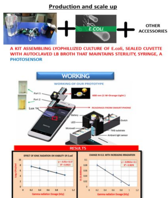
Fig. 4 Image of the gadget, its working principle and standard graphs plotted after research to estimate intensity of radiation
